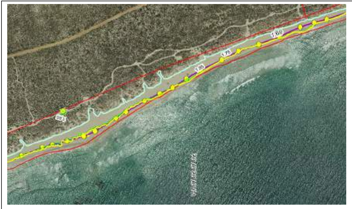
Figure 11. An illustration of the debris line waterline capture methodology developed through the MCV project.
